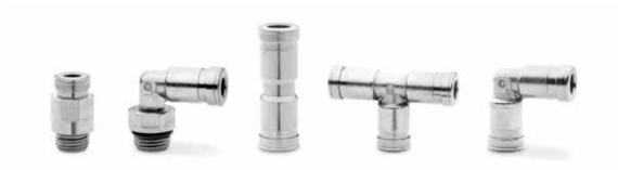
Series H8000 fittings are designed to be used in particularly dirty and dusty working environments. The patented system with double tightening on the tube guarantees a highly reliable connection and avoids any risk of leakage. The special shape of the collar prevents the entry of impurities inside the fitting, guaranteeing performance over time, retention of the tube and easy connection and release.
