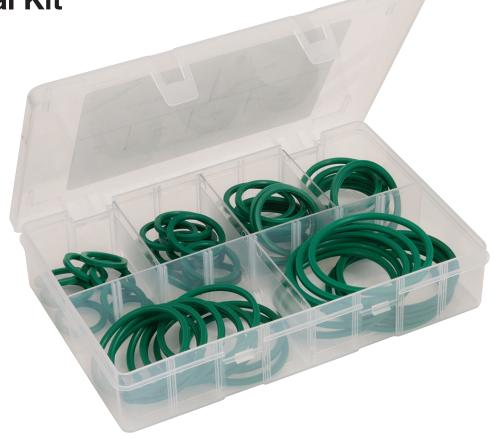
Designed to fit the SAE J518 location grooves. Made from high performance grade of polyurethane, the material provides excellent resistance-to-gap extrusion. Covers a wide temperature range from -40°C to +110°C at pressures up to 400 bar.
