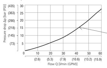
Fully open valve cross section  $P \rightarrow A$
