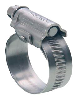
Thanks to the exclusive design of the housing, the ASFA-L W5 hose clip has excellent performance while being at the same time very compact. The cold-formed stamped band thread, smoothed on the underside, combined with bevelled band-edges protects the hose from damage.
