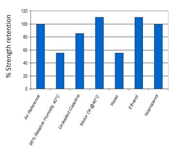
Specimens were immersed for 1000 hours at 22  $^{\circ}\mathrm{C}$  (unless otherwise stated)
