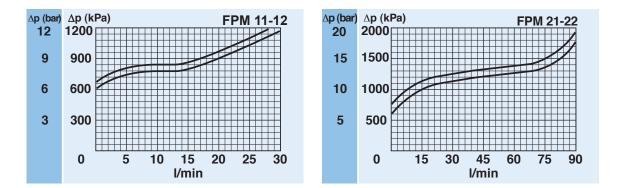
N.B. All the curves have been obtained with mineral oil having a kinematic viscosity 30 cSt and specific gravity 0,9 kg/dm<sup>3</sup>; for fluids with different features, please consider the factors described in the first part of this catalogue. All the curves are obtained from test done at the UFI HYDRAULIC DIVISION Laboratory, according to the specification ISO 3968:2005. In case of discrepancy, please check the contamination level, viscosity and features of the fluid in use.
