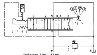
Stroke to pos. 1 (pull) - 8,5 mm Stroke to pos. 2 (push) - 5,5 mm "High force mode" Stroke to pos. 3 (push) - 5,5 + 5 mm "High speed mode"
