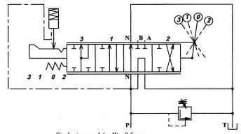
Stroke to pos. 1 (pull) - 8,5 mm Stroke to pos. 2 (push) - 5,5 mm "High force mode" Stroke to pos. 3 (push) - 5,5 + 5 mm "High speed mode"
