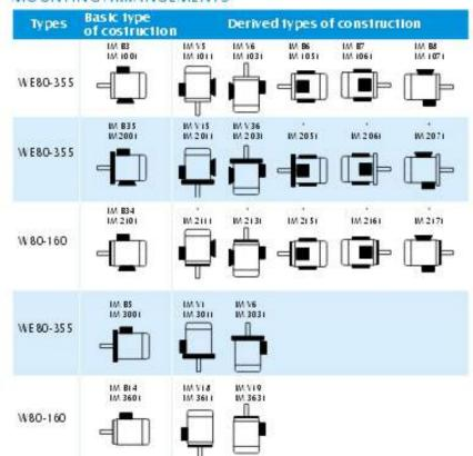
basic types of construction may be used in all derived types of construction (\*)not-defined mounting by IEC 60034-7
