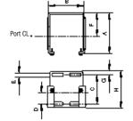
Provides secure wall mounting for individual Excelon products\* \*Except P72, P74, T73 and T74 units.
