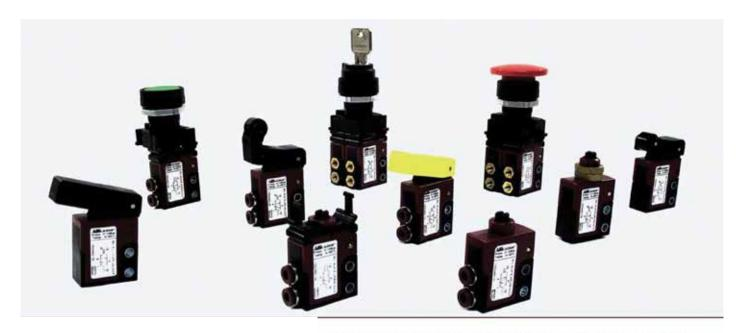
Line 100 poppet Microvalves are available in a wide range of versions and actuations in order to meet the most demanding applications requirements. Reduced dimensions, speed and signal precision represent some of the features of this Line, that can be supplied both with M5 connections and push-it fittings for pipe 4 mm, in the version with rear ports or side ports.
