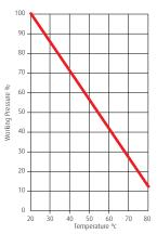
Max. recommended continuous working temperature = 70°c
